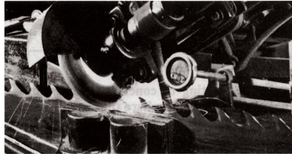
Illustration 13 – Sharpening teeth (saw gumming) on a large band saw
